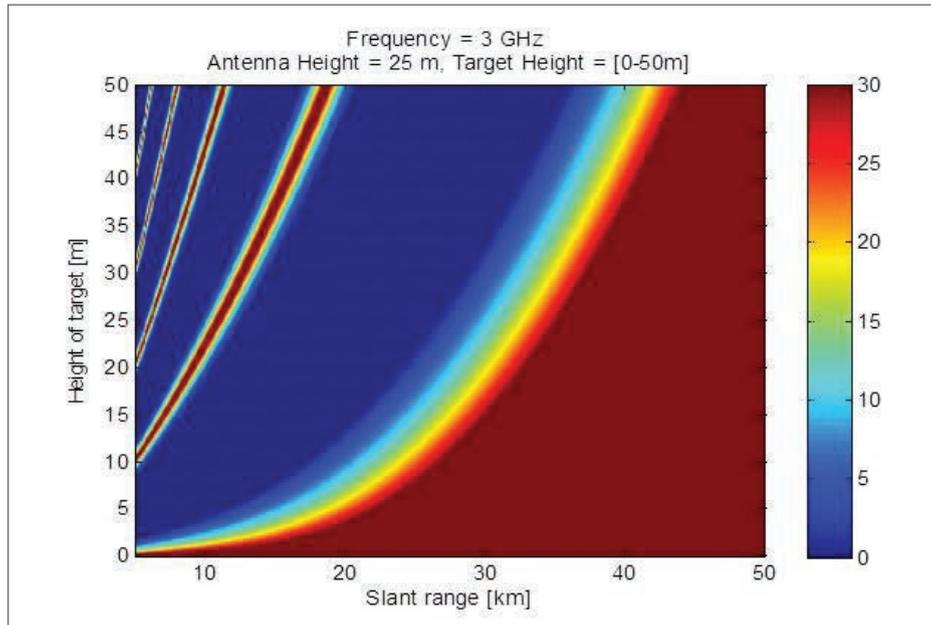
Figure 5. Propagation losses in dB due to multipath effects
