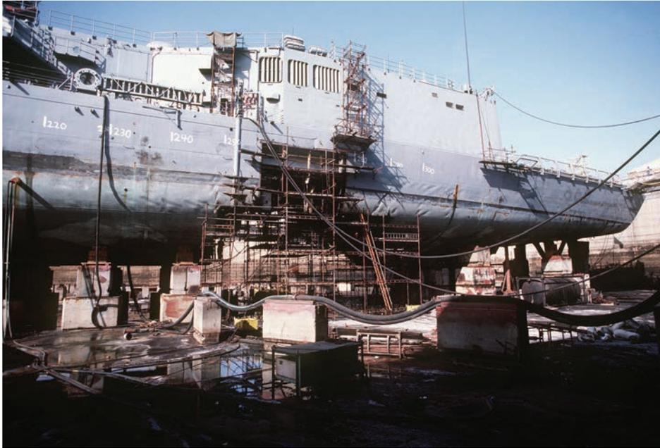
Figure 2. The eight-metre hole in the hull of guided missile frigate USS Roberts caused by an Iranian M-08 mine (© Mussi / File:Ffg58minedamage2.jpg / U.S. Navy / ID:DNST8902266 / Public Domain)
