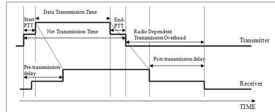
Figure 4. Process of data transmission and receipt
