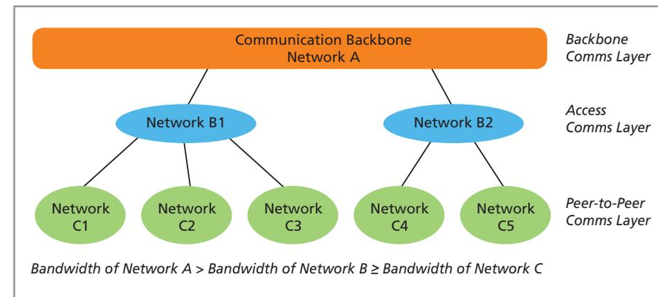
Figure 7. Hierarchical architecture of a communication network
