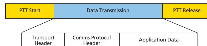
Figure 5. Simplified illustration of MTU
