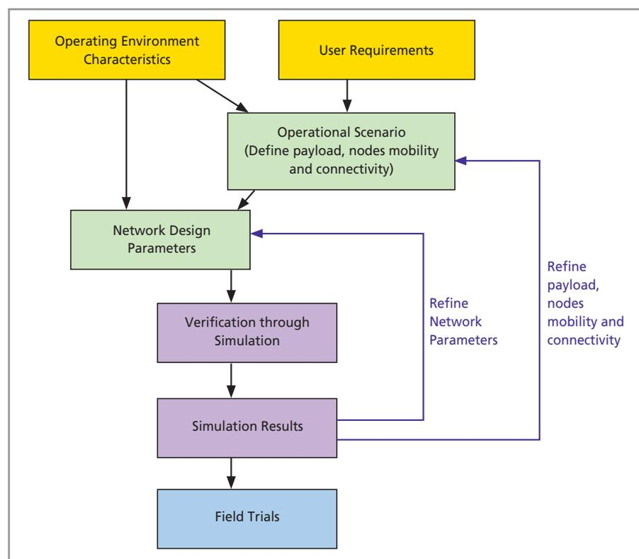
Figure 2. Proposed network design verification process
