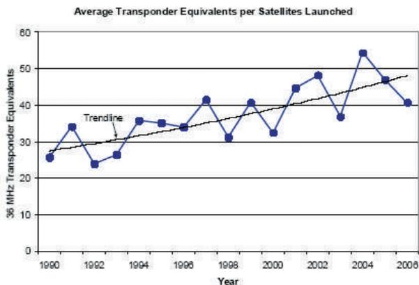
Figure 2. Average transponder equivalents per satellite launched (Futron, 2004)
