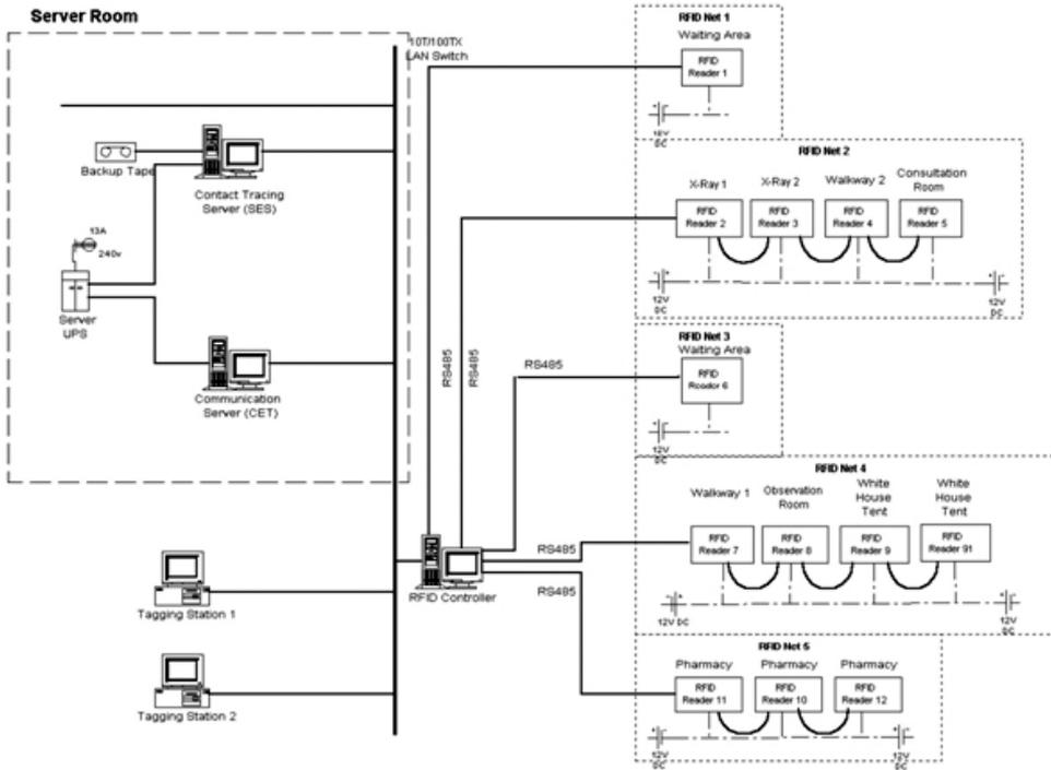
Figure 3. System deployment diagram
