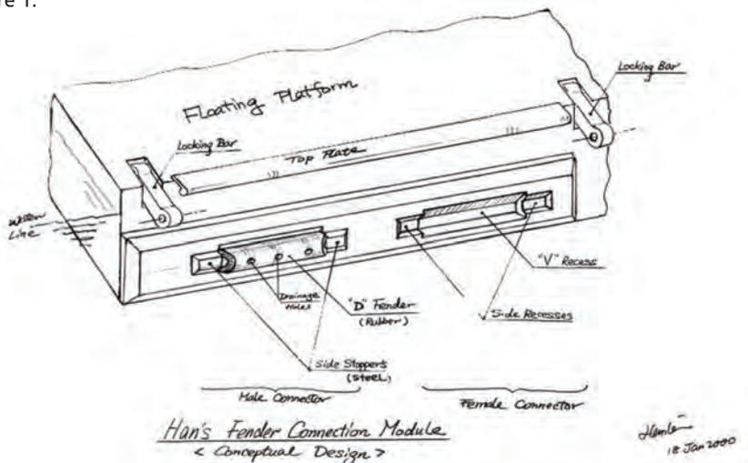
Figure 1. Fender connection module
