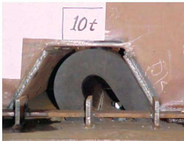
Figure 7. Full-scale load test of fender
