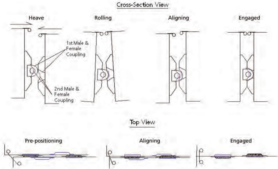
Figure 2. Fender connectors engagement in progress
