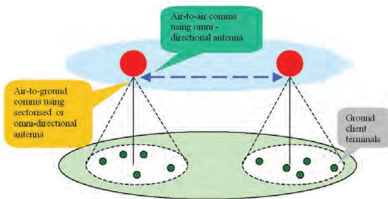
Figure 4. Two-tier communications architecture network configuration
