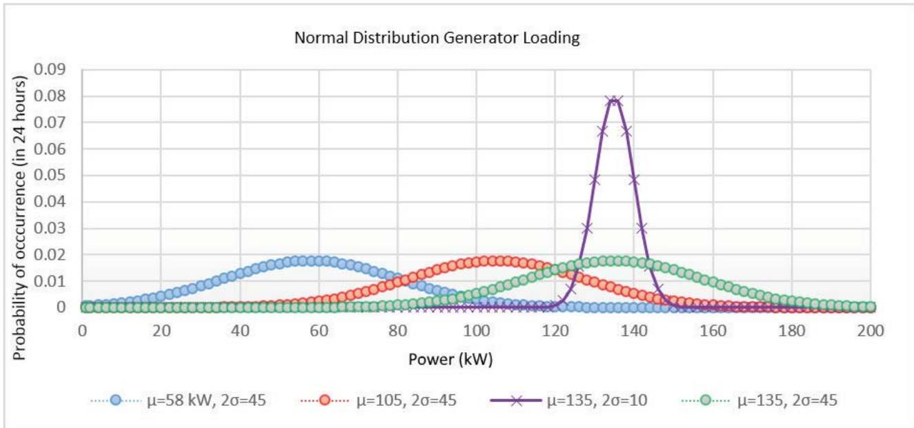
Figure 8. Normal distribution plot for generator loading curve for (a)  $\mu=58\text{kW}, 2\sigma=45$ , (b)  $\mu=105, 2\sigma=45$  (c)  $\mu=135, 2\sigma=10$  and (d)  $\mu=135, 2\sigma=45$
