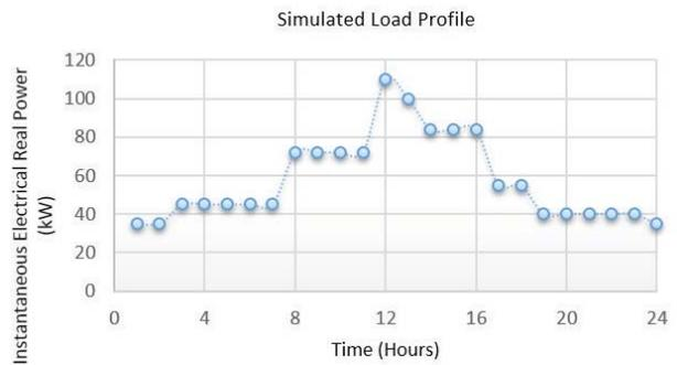
Figure 5. Simulated loading on the diesel generator
