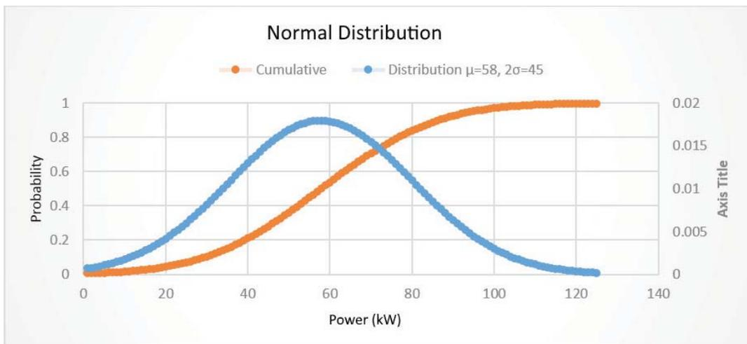
Figure 6. Simulated loading on the diesel generator with normal distribution  $\mu=58\text{ kW}$ ,  $2\sigma=45\text{ kW}$
