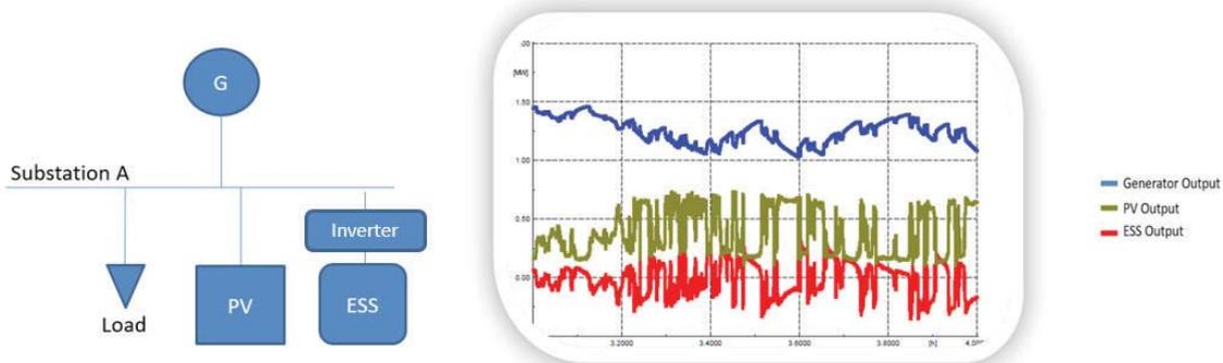
Figure 2. Microgrid with PV and ESS system, stable generator output
