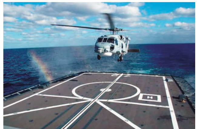
Figure 7. Deck markings for HIFR-capable ships (Ministry of Defence [MINDEF], 2018)
