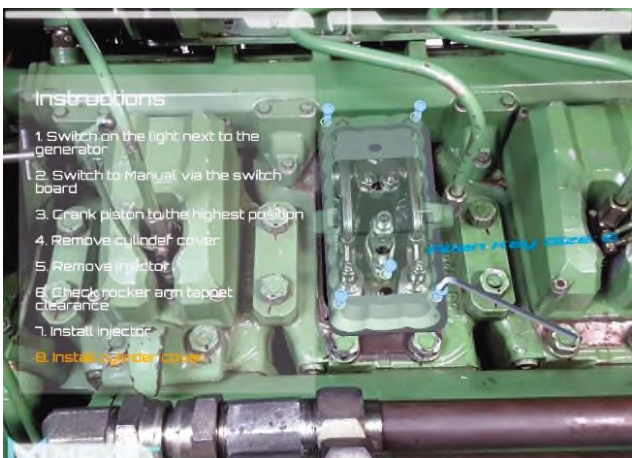
Figure 9. Screenshot of animated instructions of cylinder head cover removal
