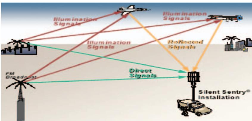
Figure 7. Passive radar concept of operation using FM broadcast (Griffiths, 2003)
