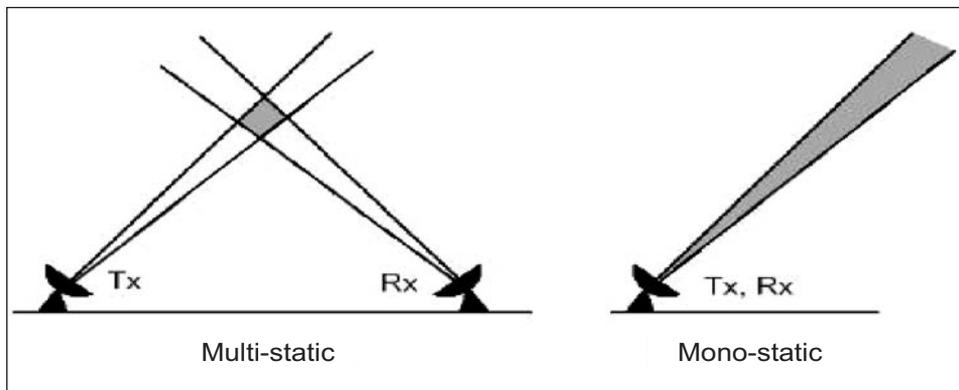
Figure 4: The transmitter and receiver are co-located for a mono-static radar, but are positioned separately in multi-static configuration. (Dravidis, 2003)
