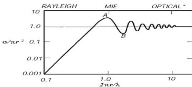
Figure 2. Normalised RCS of conducting sphere<sup>2</sup>
