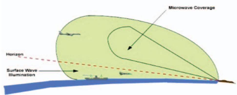
Figure 8. Coverage comparison between microwave and HFSW radars (Daronmont Technologies)
