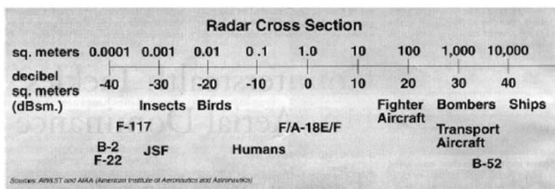
Figure 1. Examples of radar cross-sections at microwave frequencies<sup>1</sup>
