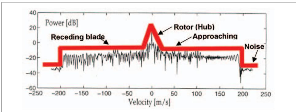
Figure 10. HERM spectrum of a hovering helicopter (Bullard, 1991)
