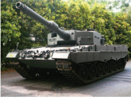
**The Leopard 2A6, with the new Rheinmetall 120mm L55 gun.** *The Leopard tank is an acquisition by DSTA on behalf of MINDEF as part of its defence procurement. (Photo: Krauss-Maffei Wegmann GmbH)*
