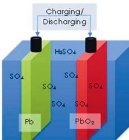
Figure 6. Operation of a lead-acid battery
