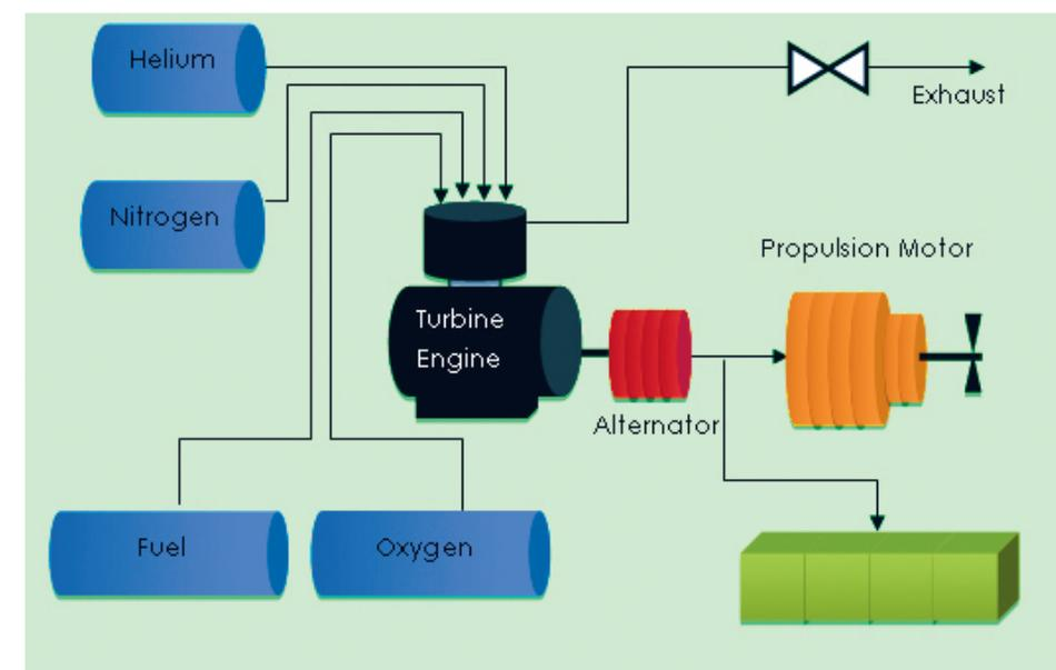
Figure 8. The Stirling AIP system
