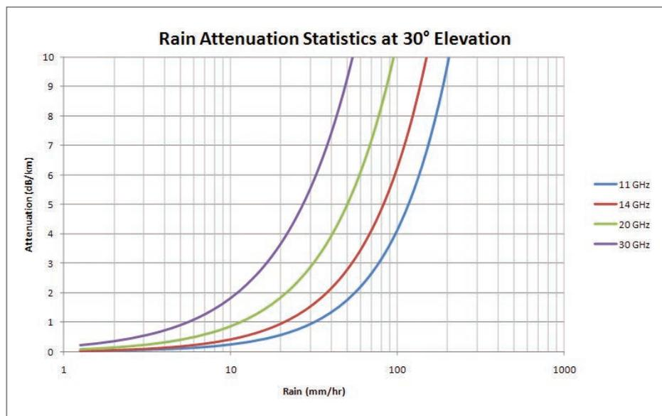
Figure 1. Rain attenuation statistics at 30 degrees elevation
