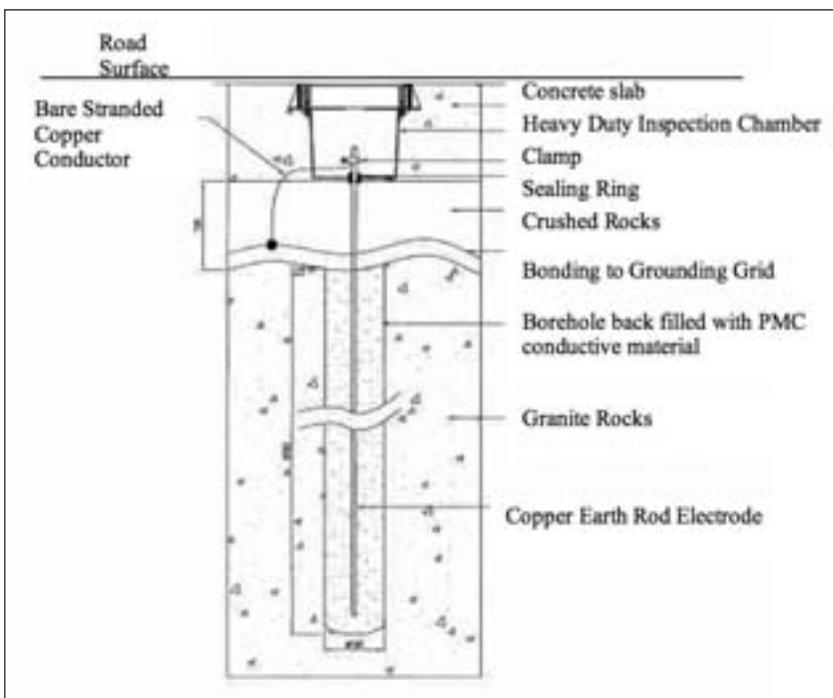
Figure 7. Illustration of a ground electrode installation in high-resistive rocks
