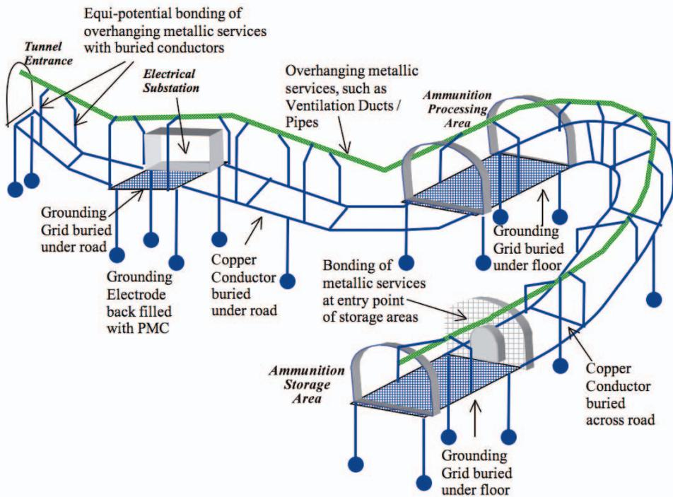
Figure 5. Illustration of grounding system for an underground ammunition facility
