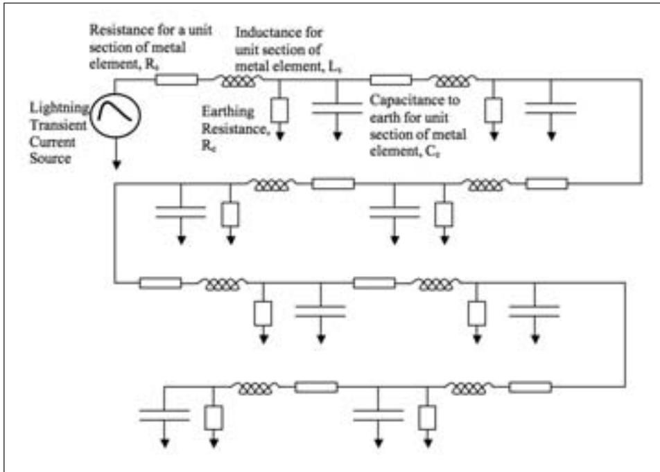
Figure 3. Circuit model of metallic element along the tunnel
