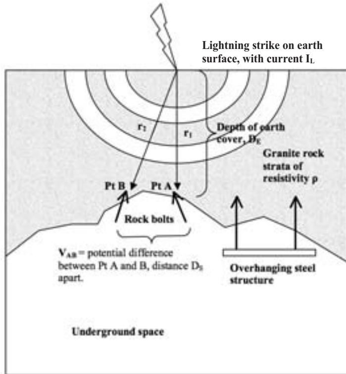
Figure 2. Illustration of lightning propagation into underground space
