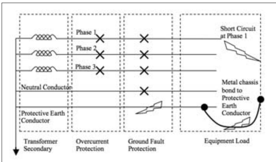
Figure 4. Illustration of a TN-S electrical earthing system
