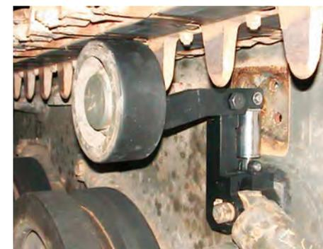
Figure 6. Isolated support roller
