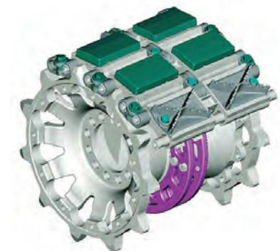
Figure 7. Double pin track around sprocket (Source: Astrum)
