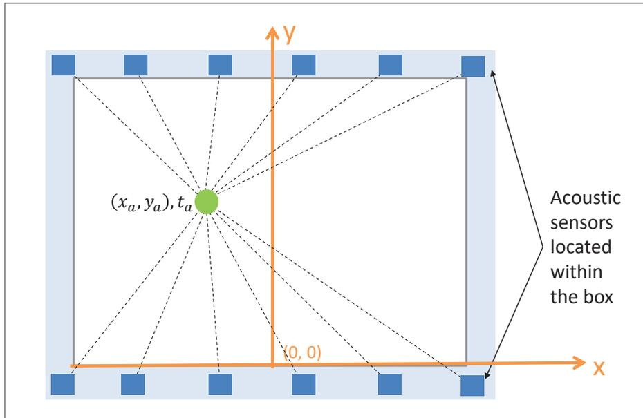
Figure 6. Coordinates of shot  $(x, y)$  determined by extrapolation of shockwaves/sound detected by the sensors
