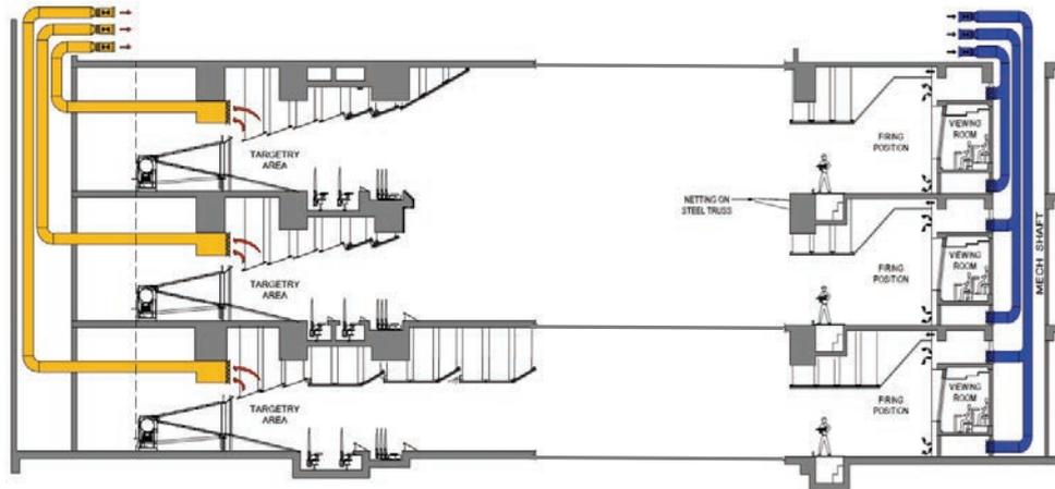
Figure 14. Schematic of range ventilation system
