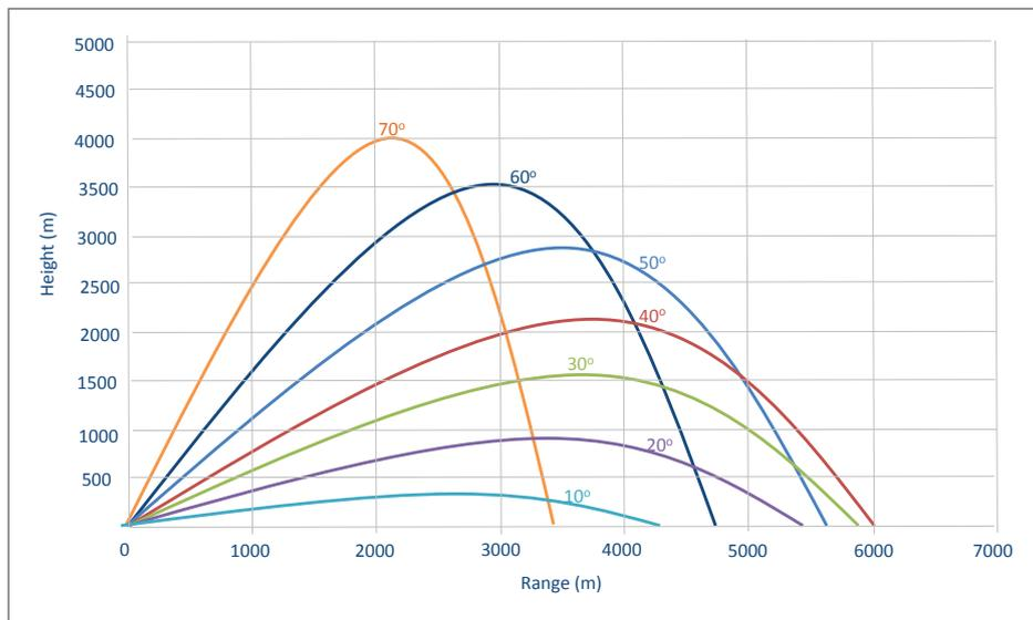
Figure 3. An example of a ballistic table
