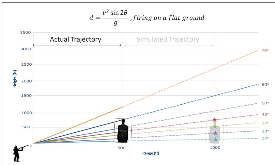
Figure 7. Simulating trajectory of a bullet beyond the physical distance
