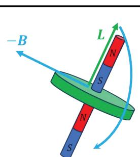
**B** is the Magnetic field applied **L** is the Angular momentum of Gyroscope **M** is the magnetic dipole moment
