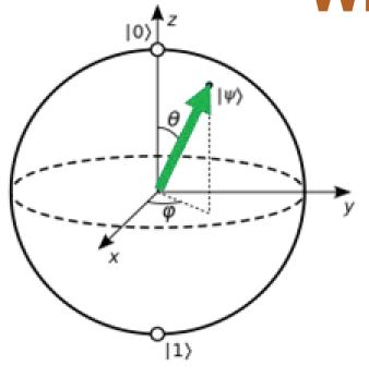
Qubits are basic units of quantum information found in the form of a two-state quantum-mechanical system
