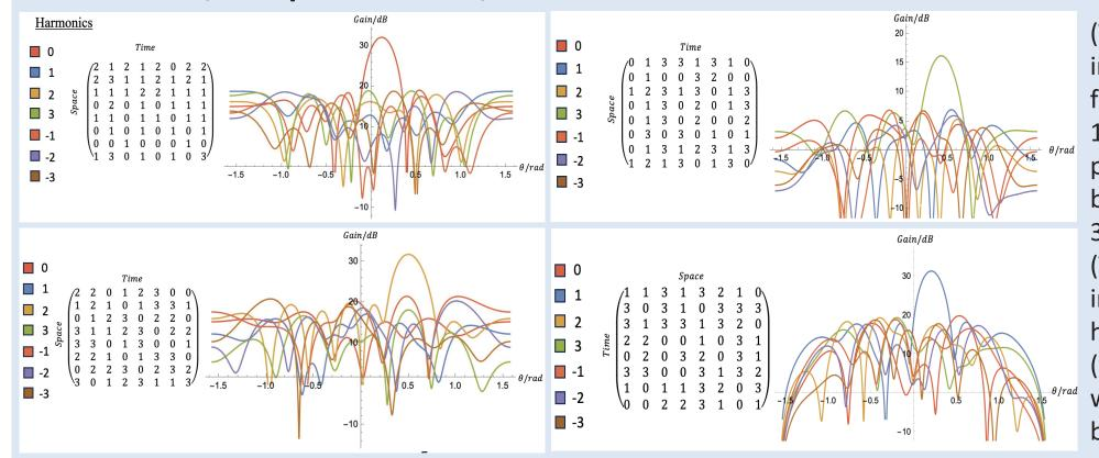
(Top-L) Normal plane wave incidence, steer beam of fundamental frequency to 10° (Bottom-L) Normal plane wave incidence, steer beam of 2<sup>nd</sup> harmonic to 30°
