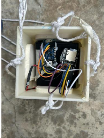
Fig 3.3f Wiring of Arduino with SD card module
