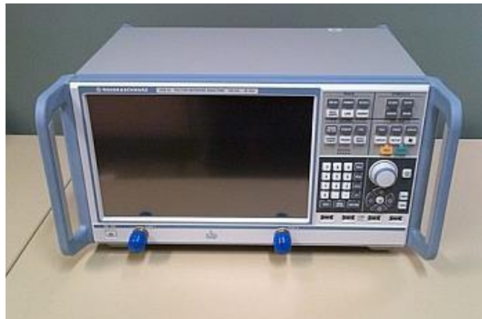
Fig. 4 (page 7-8): Rohde and Schwarz ZNB20 Vector Network Analyzer used to measure S11 of fabricated antenna
