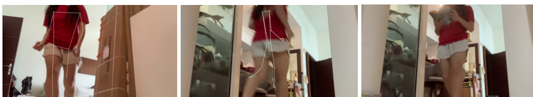
Figure 12. Accurate landmark detection with face occluded (left) | Misidentification of landmarks with face occluded (middle) | No landmarks detected with face occlusion (right)
