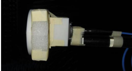
Fig. 13 Side view of setup of antenna and lens at 30mm distance apart
