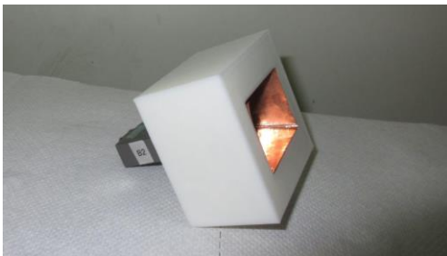
Fig. 2 3D printed antenna flare and WR90 waveguide
