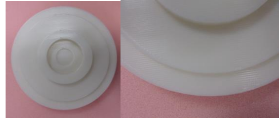
Fig. 4 Picture and close up of 3D printed microwave lens with triangular infill at 66% density and 0.6mm top and bottom sections of 100% infill density
