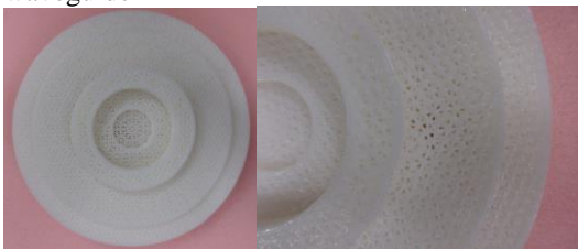
Fig. 3 Picture and close up of 3D printed microwave lens with triangular infill at 66% density
