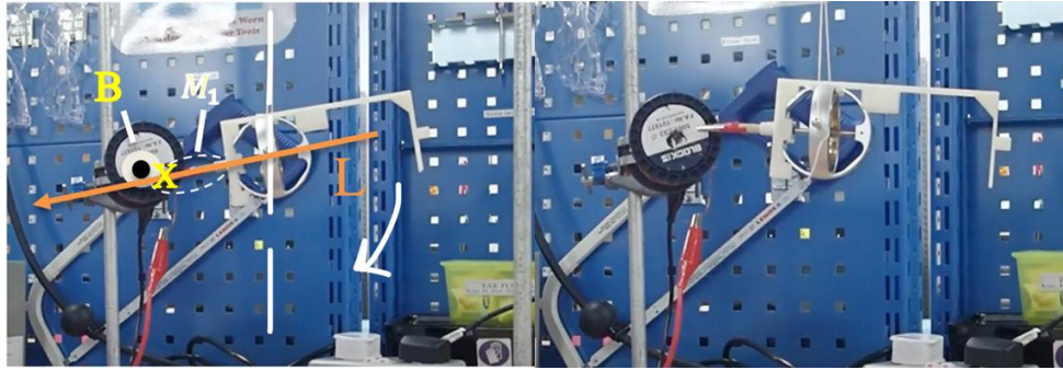
Figure 4.3: Homemade solenoids used to control gyroscopic precession (Left refers to earlier time, Right refers to observation after 1.0s)
