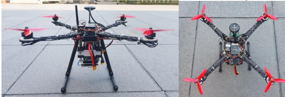
Fig 5. Physical Arrangement of Electronics on Quadcopter Frame. PM Sensor and RPI3 attached below
