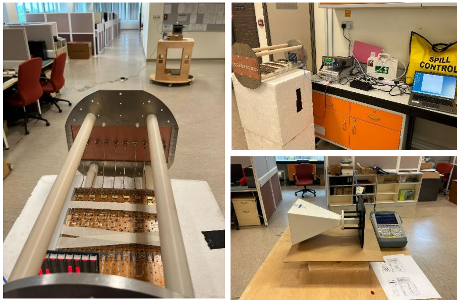
Fig 8.1.1: Experimental set-up in office space. (L) Complete view of setup. (Top-R) View of STM array and its RF backend, power supply and controller. (Bottom-R) Receiving end with receive horn connected to spectrum analyser.
